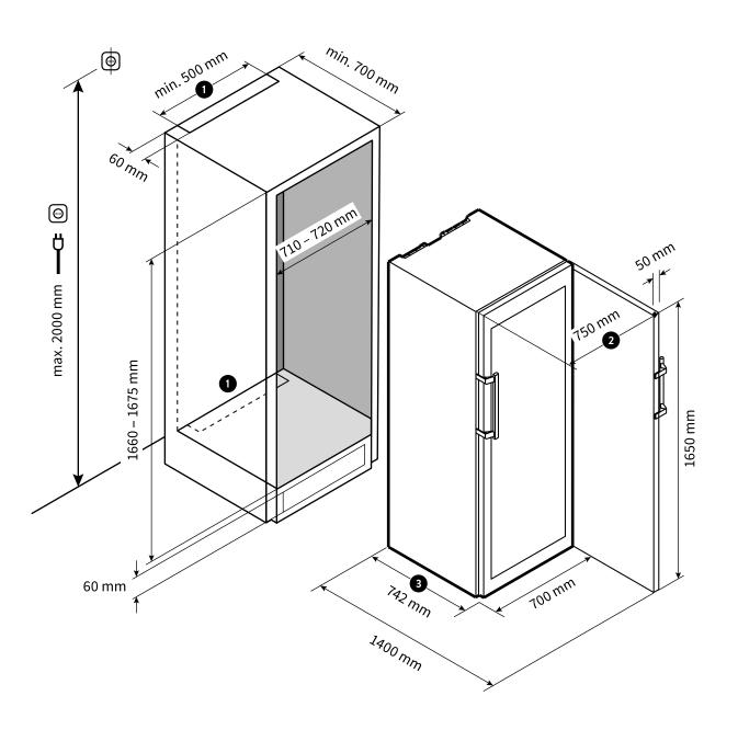
• Ventilation shaft is mandatory. **Minimum size: 300cm<sup>2</sup>**. Also possible on the side or on the back wall.
