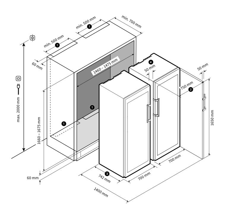
• Ventilation shaft is mandatory. **Minimum size: 300cm<sup>2</sup>**. Also possible on the side or on the back wall.
