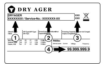
When contacting customer service, provide the type designation 1 the service number 2, the service index 3 and the serial number 4 on the type plate.
