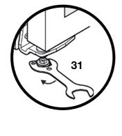
**31.** Place the unit in its final position at the installation location. Unscrew the adjustable foot at the lower hinge angle until it rests on the floor, then continue to rotate 90°.
