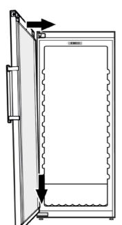
27. Place the door on the bolt and guide it to the hinge bracket at the top.
