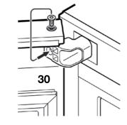
**30.** Unscrew the screw from the bearing pin and screw it into the hole in the hinge bracket.
