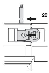
**29.** Insert the bearing bolt until the groove of the bolt is in line with the bore of the hinge bracket.
