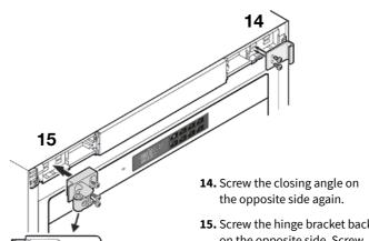
**15.** Screw the hinge bracket back on the opposite side. Screw 3 screws into the marked openings.
