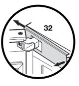
**32.** Disengage the cover on the inside and slide it outwards.
