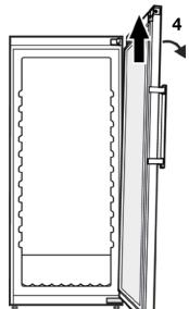
**4.** Slightly tilt the door to the side and remove it upwards.
