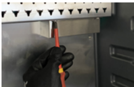
5. Unscrew the cover with a Phillips screwdriver.
