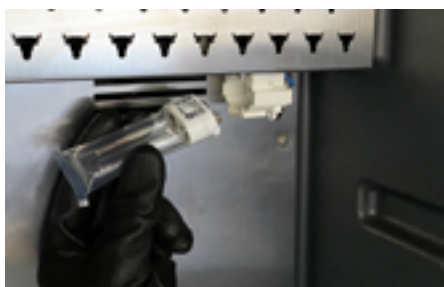
7. Pull out the old UVC bulb carefully then carefully insert the replacement UVC bulb. Do not remove the outer plastic cover of the UVC replacement bulb.
